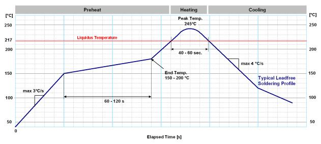
Figure 31: Recommended soldering profile
