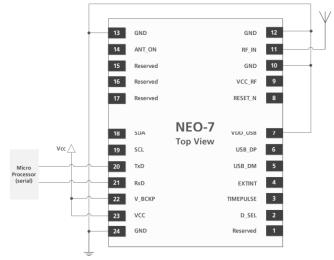
Figure 5: NEO-7 passive antenna design
