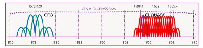
Figure 27: GPS & GLONASS SAW filter
