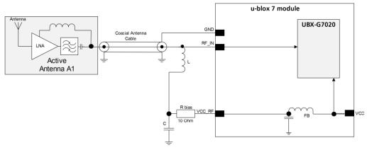
Figure 19: Active antenna design, external supply from VCC\_RF
