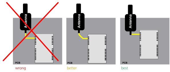
Figure 14: Recommended micro strip routing to RF pin
