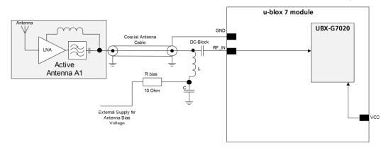
Figure 20: Active antenna design, direct external supply
