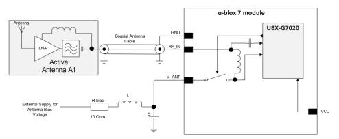
Figure 23: Module design with active antenna, external supply
