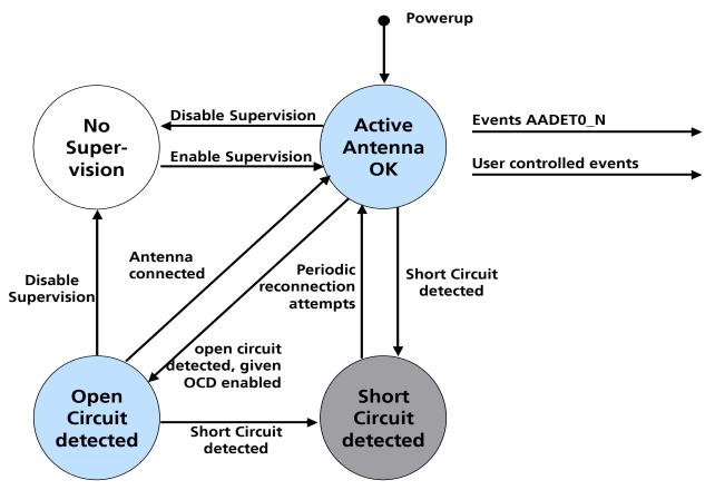
Figure 21: State diagram of active antenna supervisor
