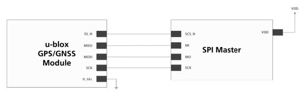
Figure 4: Connecting to SPI Master
