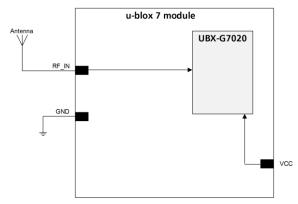
Figure 17: Module design with passive antenna
