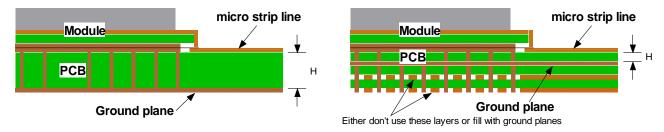
Figure 13: PCB build-up for micro strip line. Left: 2-layer PCB, right: 4-layer PCB
