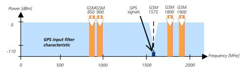
Figure 37: Out-band jamming signals
