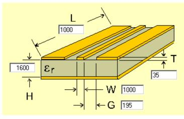
Figure 15: Micro strip on a 2-layer board (Agilent AppCAD Coplanar Waveguide)
