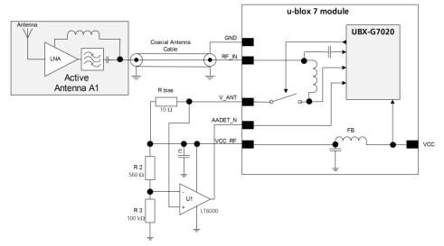
Figure 24: Schematic of open circuit detection
