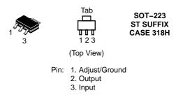
Heatsink tab is connected to Pin 2.
