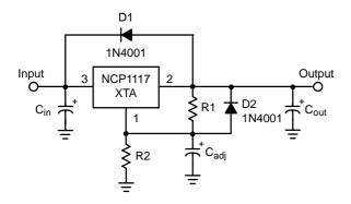
Figure 22. Protection Diode Placement
