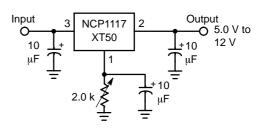
Figure 29. Adjusting Output of Fixed Voltage Regulators
