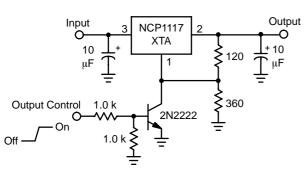
$V_{out(Off)} = V_{ref}$
