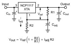
Figure 21. Adjustable Output Regulator
