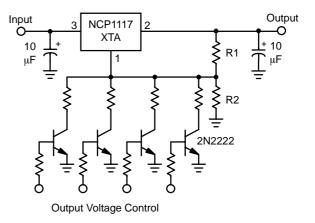
Resistor R2 sets the maximum output voltage. Each transistor reduces the output voltage when turned on.
