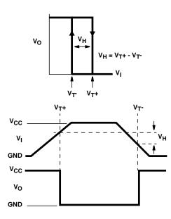
FIGURE 3. HYSTERESIS DEFINITION, CHARACTERISTIC, AND TEST SETUP
